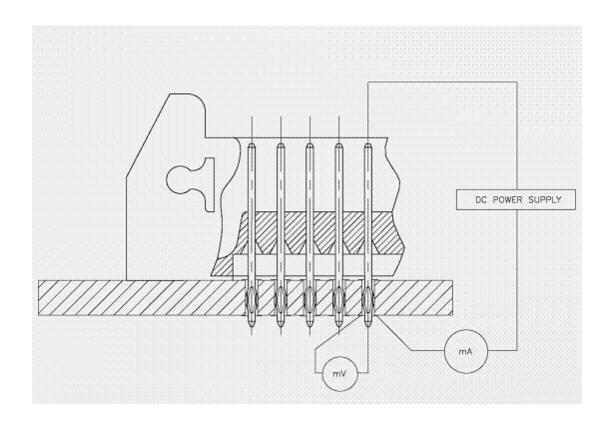
FIGURE 1 – CONTACT TO PLATED THRUGH HOLE RESISTANCE
