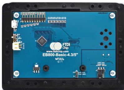
Figure 3-2 - VM800B module profile 4.3" display version
