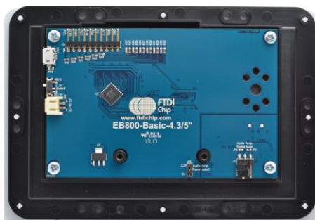
Figure 3-3 - VM800B module profile 5" display version
