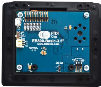
Figure 3-1 – VM800B module profile 3.5" display version
