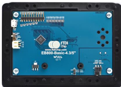
Figure 3-2 - VM800B module profile 4.3” display version
