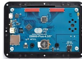
Figure 2.2 VM800P43A Module Profile 4.3" Display Version
