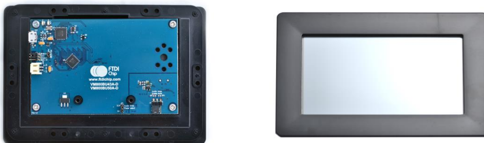
Figure 3-3 - VM800BU module profile 5" display version
