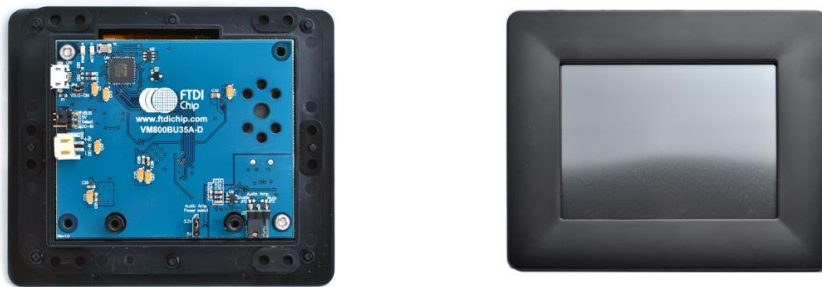
Figure 3-1 - VM800BU module profile 3.5" display version
