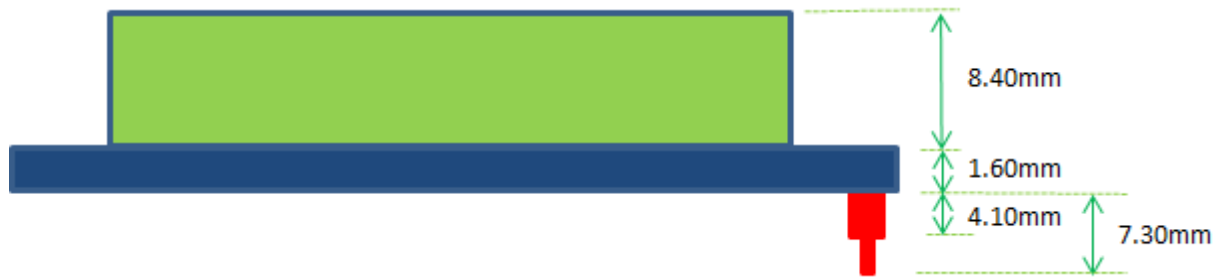
Figure 3-4 - VI800A-N485U module PCB side view
