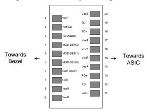
**Pinout of Connector Block on Host Board**
