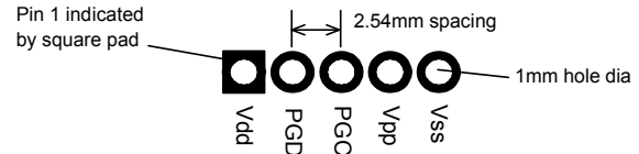
Figure 9. Recommended plate-through connector design
