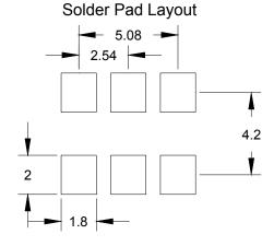
Note: XPRESSO LVDS XOs are designed to fit on Industry standard, 6 pad, layouts.
