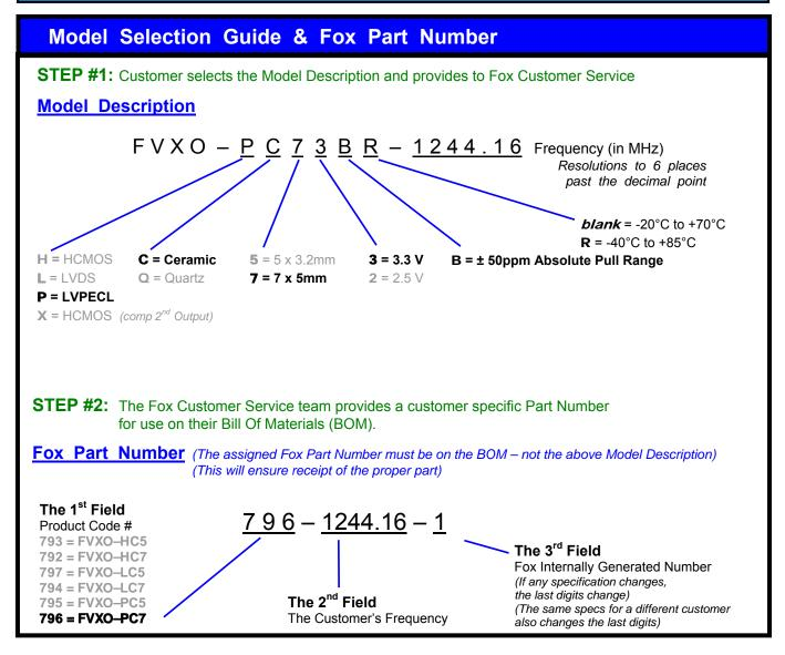
This example, FVXO-PC73BR-1244.16 = Voltage Controlled, LVPECL Output, Ceramic, 7 x 5mm Package, 3.3V, ±50 PPM Absolute Pull Range, -40 to +85°C Temperature Range, at 1244.16 MHz
