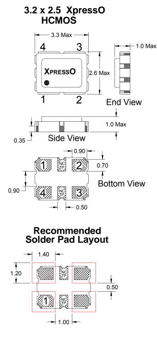
Note: XpressO HCMOS XO's are designed to fit on industry standard, 4 pad layouts.
