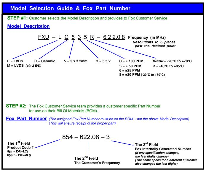
This example, FXU-LC535R-622.08 = LVDS Output, Ceramic, 5 x 3.2mm Package, 3.3V, ±50 PPM Stability, -40 to +85°C Temperature Range, at 622.08 MHz
