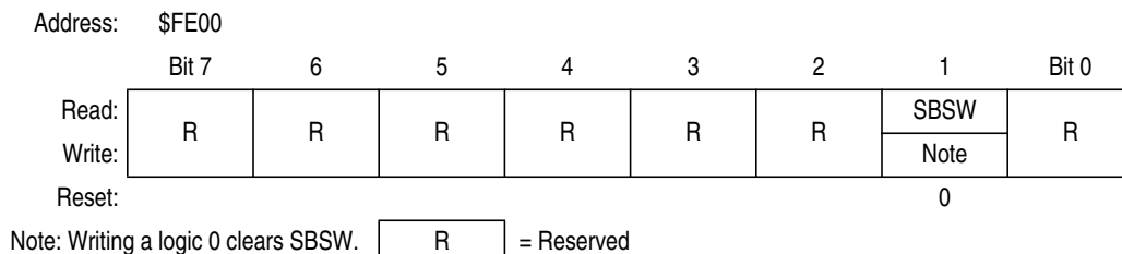
Figure 21-6. SIM Break Status Register (SBSR)
