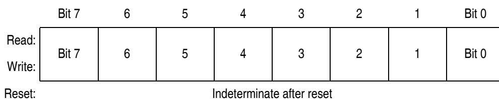
Figure 10-13. TIM Channel 0 Register Low (TCH0L)
