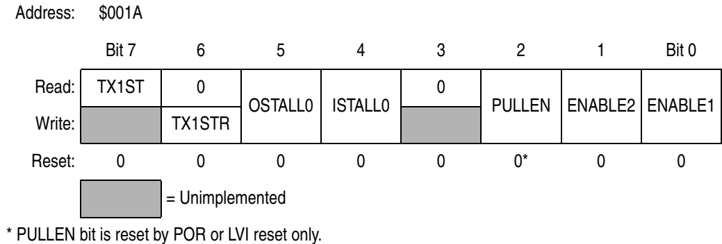
Figure 9-22. USB Control Register 3 (UCR3)
