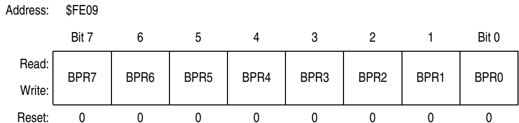
Figure 4-4. FLASH Block Protect Register (FLBPR)
