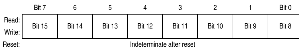
Figure 14-12. TIM Channel x Register High (TCHxH)
