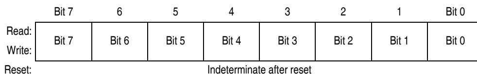
Figure 14-13. TIM Channel Register Low (TCHxL)
