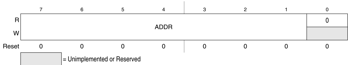
Figure 13-3. IIC Address Register (IICA)
