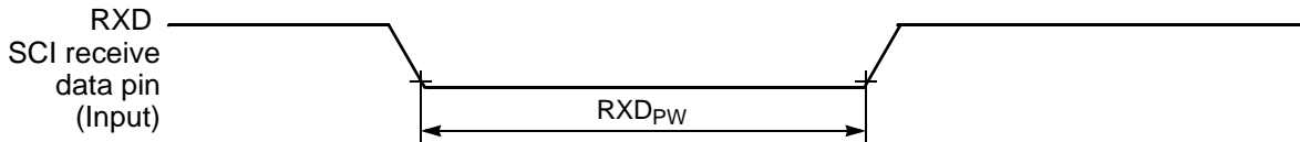
Figure 10-15 RXD Pulse Width
