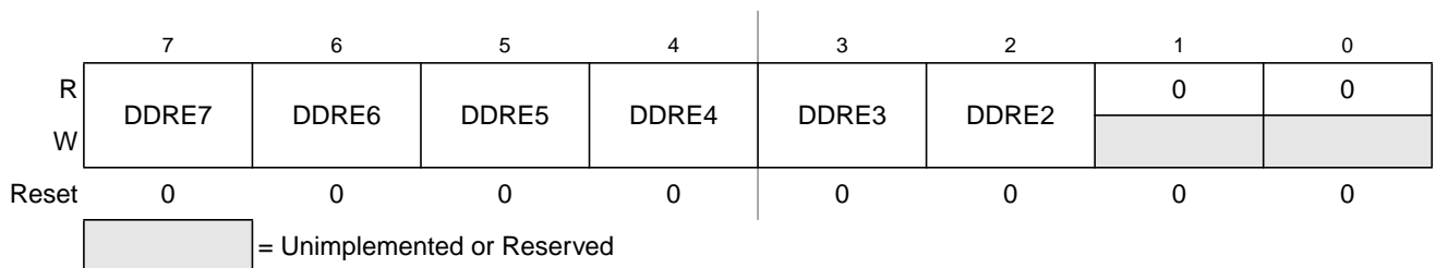
Figure 23-12. Port E Data Direction Register (DDRE)
