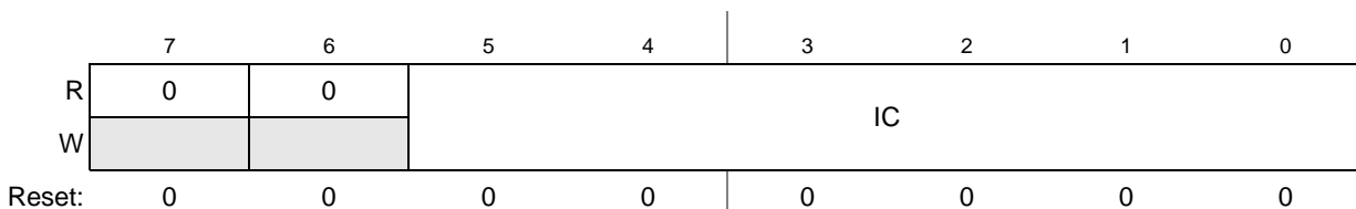
Figure 24-3. I 2 C Frequency Divider Register (I2FDR)
