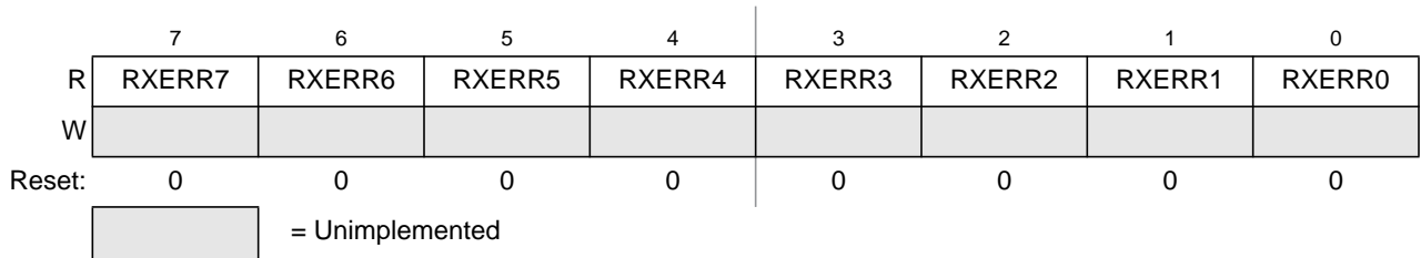
Figure 12-17. MSCAN Receive Error Counter (CANRXERR)
