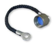
Protective covers fit Series 800 plug and receptacle connectors. Aluminum or stainless steel. Fluorosilicone rubber gasket protects connector from contamination and water ingress. Attach to panel or cable with a variety of lanyards and fittings. Lanyard styles include braided nylon rope, stainless steel wire or sash chain. Stainless steel wire available with flexible, rugged polyurethane coating or Fluoropolymer sleeve for high temperature requirements.
