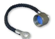
Protective covers fit Series 800 plug and receptacle connectors. Aluminum or stainless steel. Fluorosilicone rubber gasket protects connector from contamination and water ingress. Attach to panel or cable with a variety of lanyards and fittings. Lanyard styles include braided nylon rope, stainless steel wire or sash chain. Stainless steel wire available with flexible, rugged polyurethane coating or Fluoropolymer sleeve for high temperature requirements.
