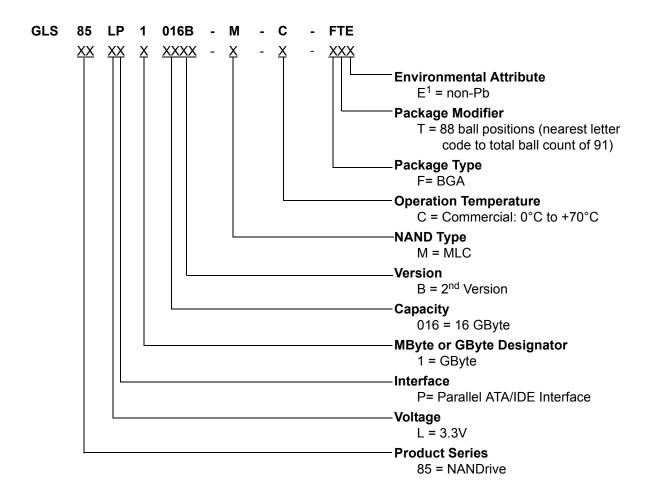
Environmental suffix "E" denotes non-Pb solder. GLS non-Pb solder devices are "RoHS Compliant".
