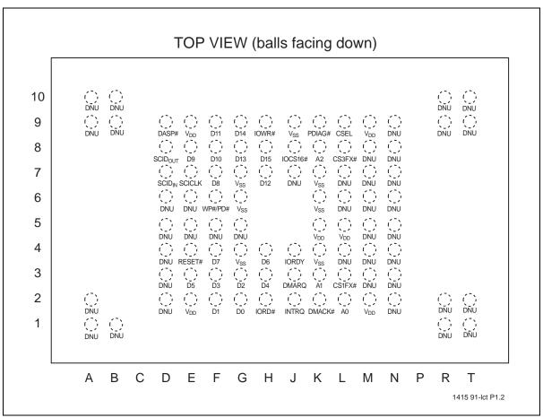
Figure 2: Pin Assignments for 91-Ball BGA
