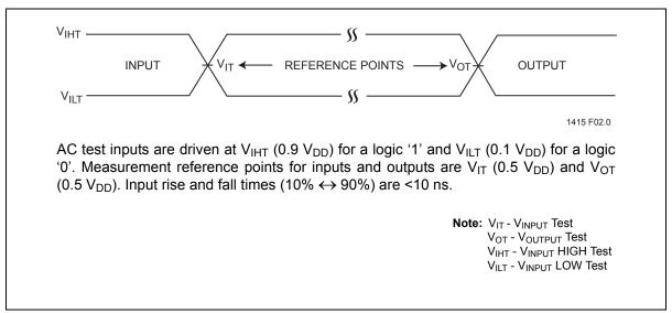
Figure 4: AC Input/Output Reference Waveforms
