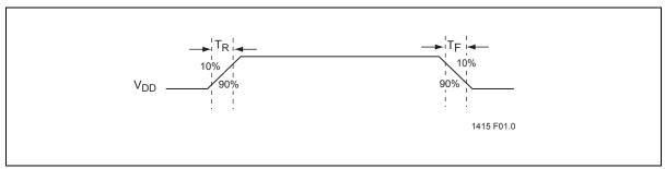
Figure 3: Power-on and Brown-out Reset Timing
