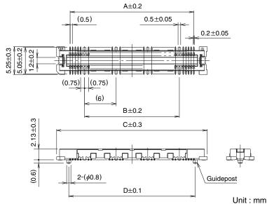
No. of Contacts Part No. HRS No. D RoHS Α В С Ε Remarks Ground Signal FX11A-60P/06-SV(71) 573-0502-0 71 60 6 17.5 12 22.6 18 19.4 25.5 FX11A-80P/08-SV(71) 573-0503-2 71 80 8 23.5 28.6 31.5 18 24 25.4 With guideposts 573-0504-5 71 100 37.5 FX11A-100P/10-SV(71) 10 29.5 24 34.6 30 31.4 Yes FX11B-60P/06-SV(71) 25.5 573-0512-3 71 60 6 17.5 12 22.6 19.4 FX11B-80P/08-SV(71) 573-0513-6 71 80 8 23.5 18 28.6 25.4 31.5 Without guideposts FX11B-100P/10-SV(71) 573-0514-9 71 37.5 100 10 29.5 24 34.6 31.4
