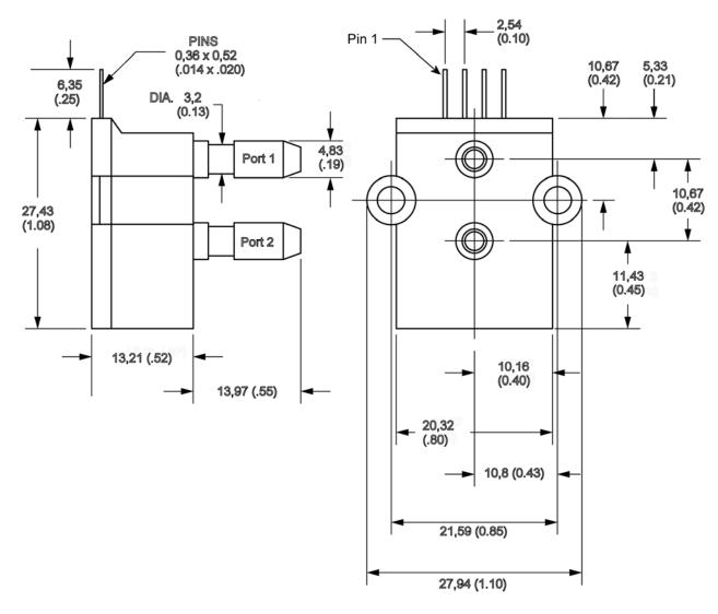
Note: For gage sensor apply pressure to port 2.
