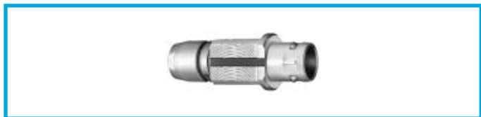
FIG Straight plug for remote handling, key (G) or keys (A...L and R), special alignment mark, knurled handling surface, cable collet
