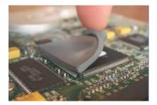
CoolZorb 400 is a hybrid absorber/thermal management material that is used for EMI mitigation. Product is used like a traditional thermal interface material between heat source such as an IC and heat sink or other heat transfer device or metal chassis. CoolZorb 400 also functions to suppress unwanted energy coupling, resonances or surface currents causing board level EMI issues.
