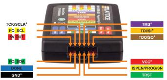
\* Indicates flywire connections required for most basic JTAG programming.
