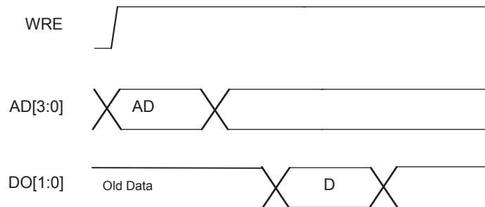
Figure 3-7. Slice Single /Dual Port Read Cycle Timing
