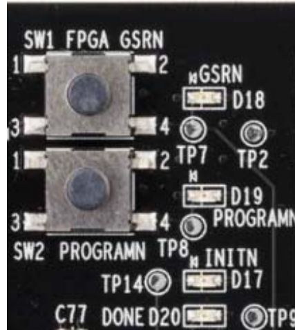
Figure 3. ECP5 Status LEDs and Push-button Controls
