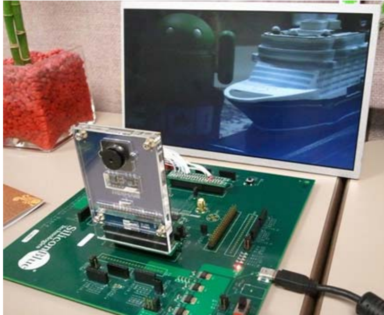
Figure 19-12. 5-Megapixel CMOS Camera to LVDS Display on iCEman40 Evaluation Board
