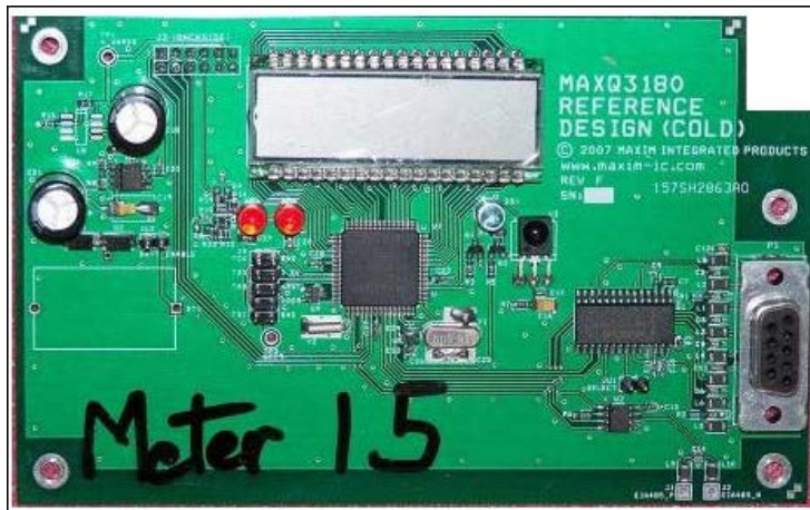
Figure 11. The cold board of the reference design.
