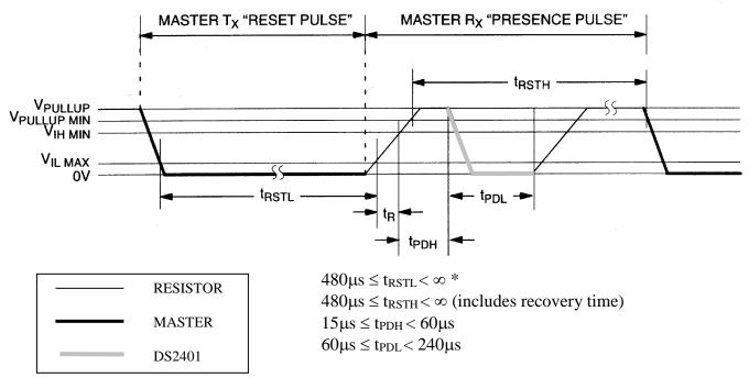
\* In order not to mask interrupt signaling by other devices on the 1-Wire bus,  $t_{RSTL} + t_R$  should always be less than 960µs.
