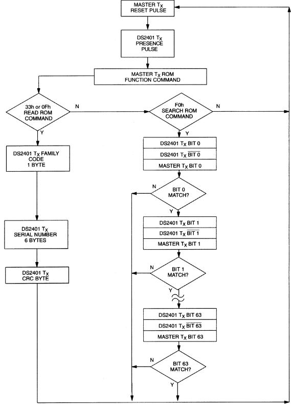
**INITIALIZATION PROCEDURE "RESET AND PRESENCE PULSES"** Figure 5
