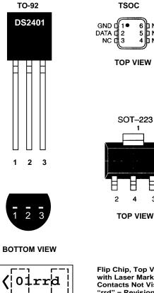
Flip Chip, Top View with Laser Mark, Contacts Not Visible. "rrd" = Revision/Date
