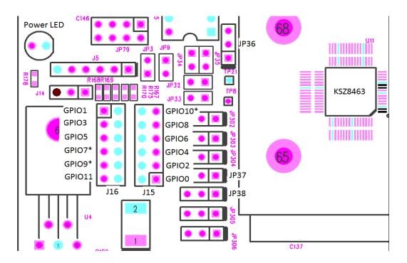
Figure 3 GPIO Connectors and Related Jumper Locations
