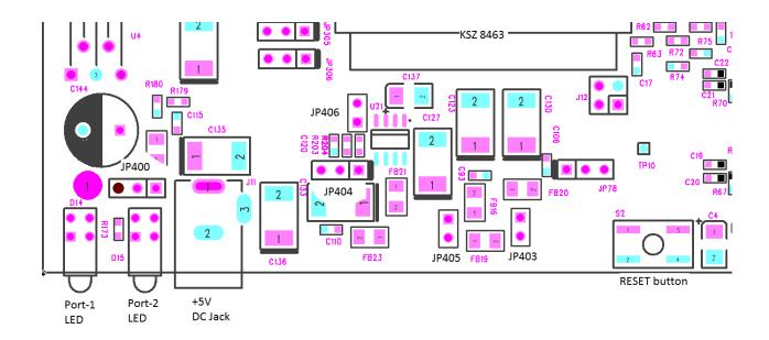
Figure 2 Power Supply Section and Related Jumper Locations
