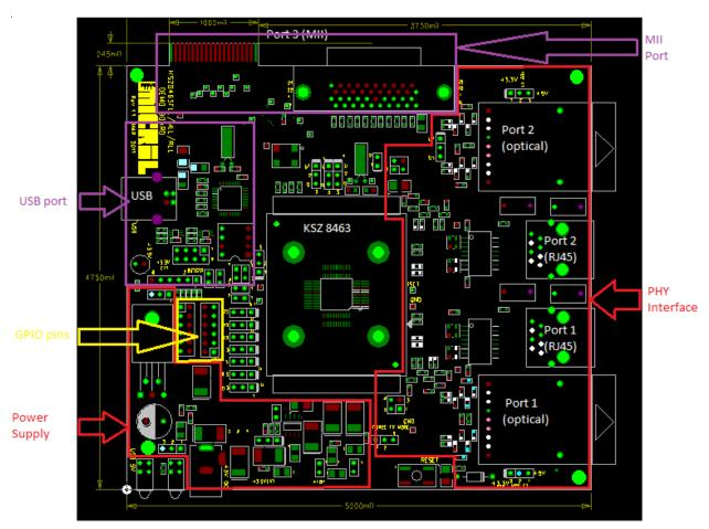
Figure 4 Topside Layout of the Board
