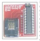
For 8-pin (PIC12F629/675), 14-pin (PIC16F630/676) or 18-pin (PIC16F627A/628A/648A) devices, limited I/O make integrated in-circuit debugging impractical. Instead, incircuit debugging is made possible by using a header containing an equivalent device with integrated incircuit debugging peripheral. For debugging, the header is connected
