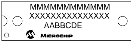
28-Lead PDIP (Skinny DIP)
