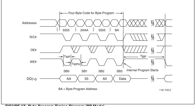
FIGURE 17: Byte-Program Timing Diagram (PP Mode)
