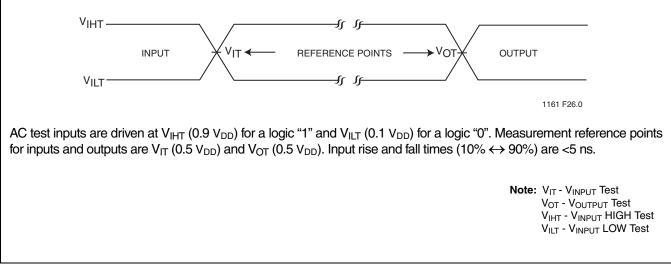
FIGURE 23: AC Input/Output Reference Waveforms (PP Mode)
