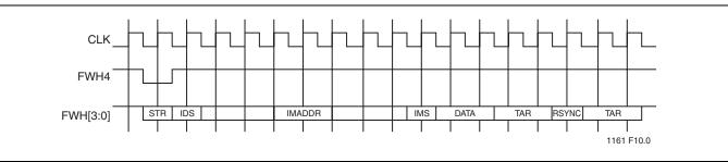
FIGURE 7: Write Waveforms
