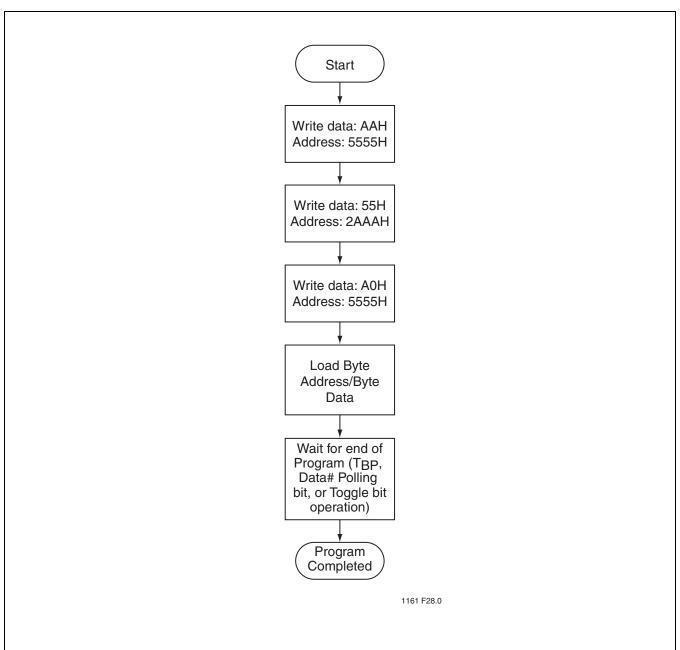
FIGURE 25: Byte-Program Algorithm
