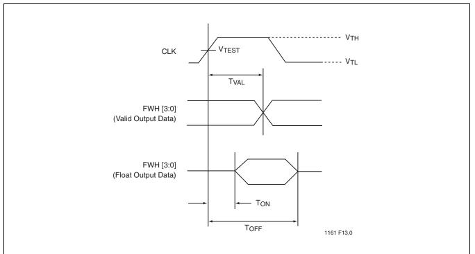
FIGURE 10: Output Timing Parameters
