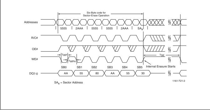
FIGURE 18: Sector-Erase Timing Diagram (PP Mode)
