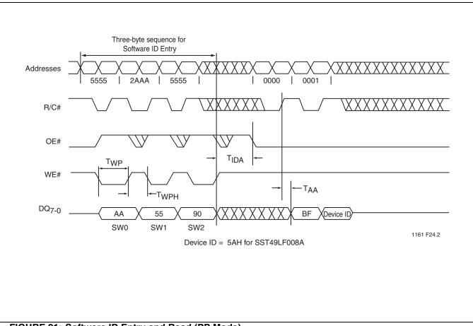
FIGURE 21: Software ID Entry and Read (PP Mode)
