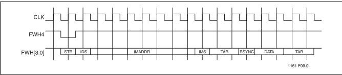
FIGURE 6: Single-Byte Read Waveforms
