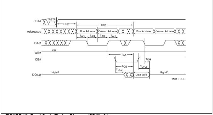
FIGURE 13: Read Cycle Timing Diagram (PP Mode)
