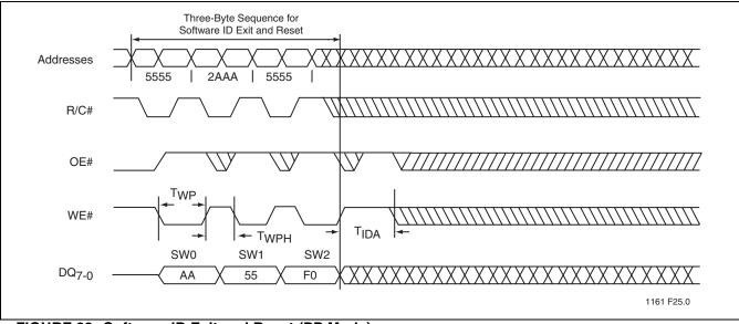
FIGURE 22: Software ID Exit and Reset (PP Mode)
