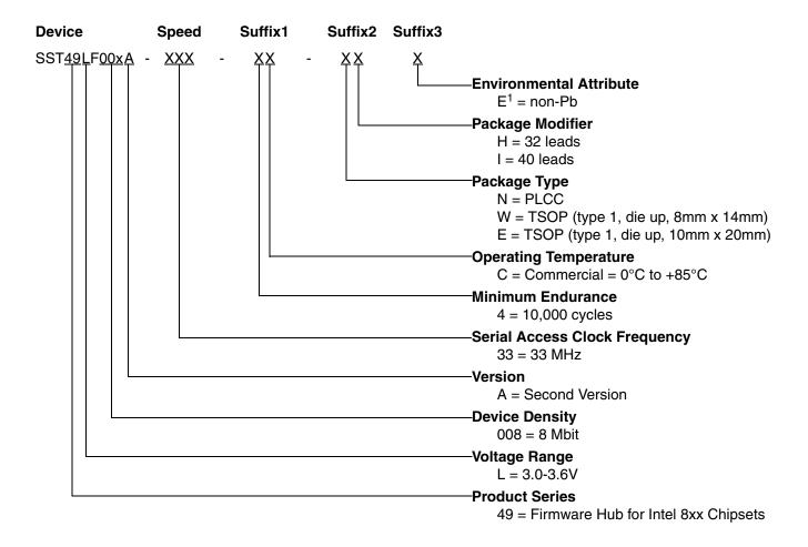
1. Environmental suffix "E" denotes non-Pb solder. SST non-Pb solder devices are "RoHS Compliant".
