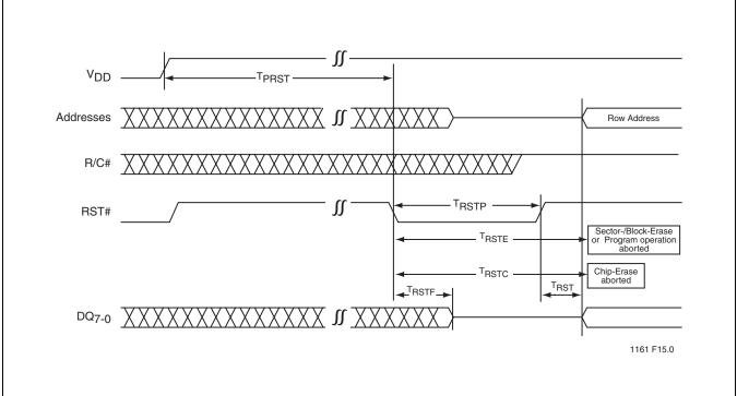
FIGURE 12: Reset Timing Diagram (PP Mode)
