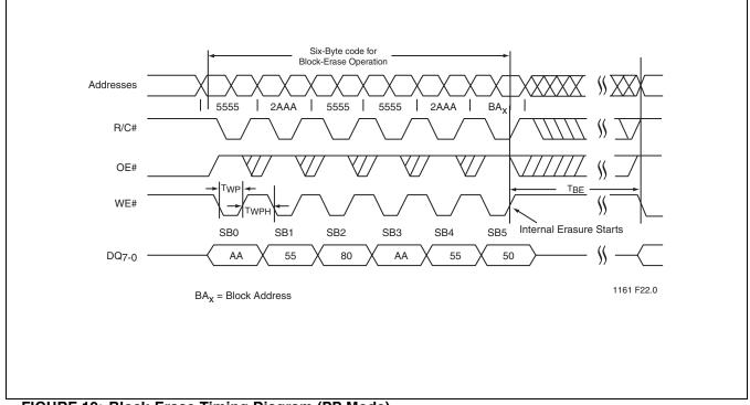
FIGURE 19: Block-Erase Timing Diagram (PP Mode)
