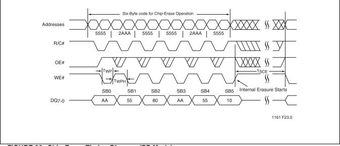
FIGURE 20: Chip-Erase Timing Diagram (PP Mode)
