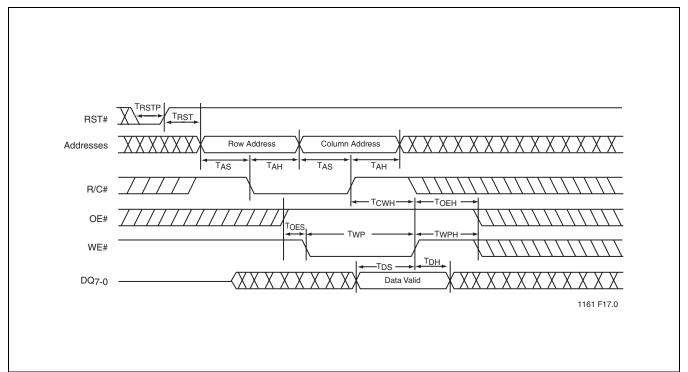
FIGURE 14: Write Cycle Timing Diagram (PP Mode)
