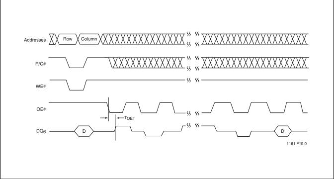
FIGURE 16: Toggle Bit Timing Diagram (PP Mode)
