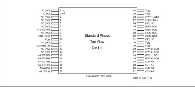
FIGURE 4: Pin Assignments for 40-lead TSOP
