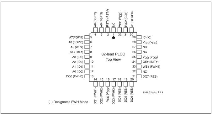
FIGURE 3: Pin Assignments for 32-lead PLCC
