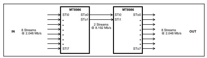
Figure 11 - 256-Channel Switch with Rate Conversion between 2.048 and 8.192 Mb/s
