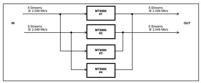
Figure 9 - 512-Channel Switch with Serial Streams at 2.048 Mb/s
