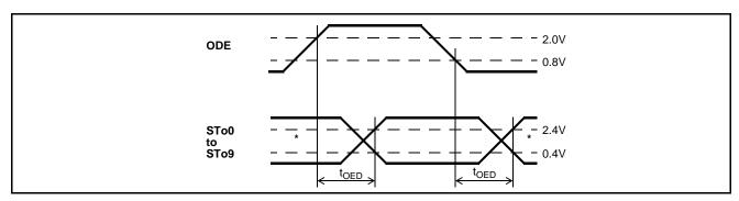
Figure 21 - Output Driver Enable for Streams at 4.096 and 8.192 Mb/s
