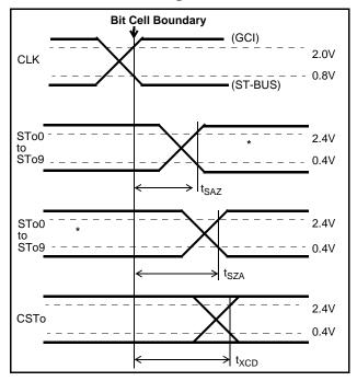
Figure 18 - Serial Outputs and External Control
