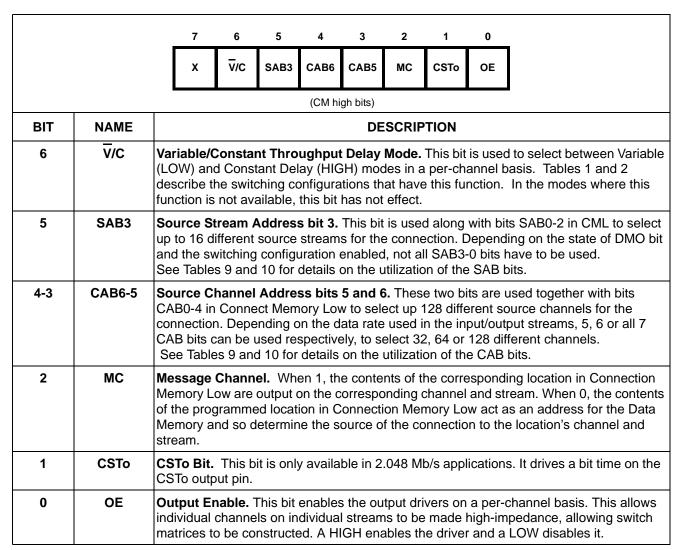
Figure 5 - Connection Memory High (CMH) Bits
