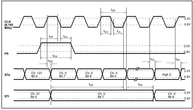
Figure 25 - Rate Conversion Mode (DMO bit=1) - 2 Mb/s to 8 Mb/s
