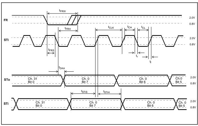
Figure 16 - ST-BUS Timing (CLKM bit=0)
