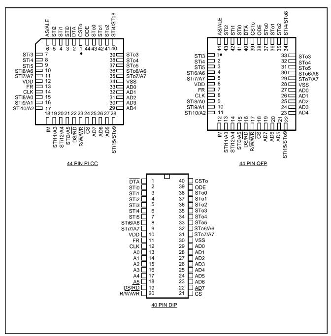
Figure 2 - Pin Connections
