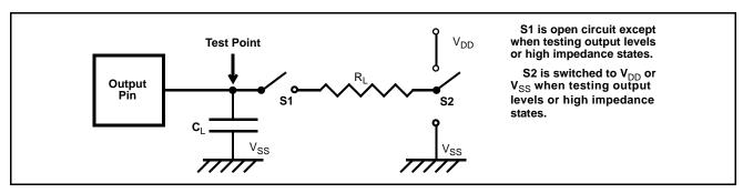
Figure 15 - Output Test Load
