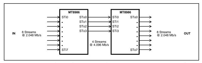
Figure 10 - 256-Channel Switch with Rate Conversion between 2.048 and 4.096 Mb/s
