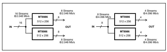
Figure 12 - 512-Channel Non-Blocking Switch Matrix with Serial Streams at 2.048 or 4.096 Mb/s
