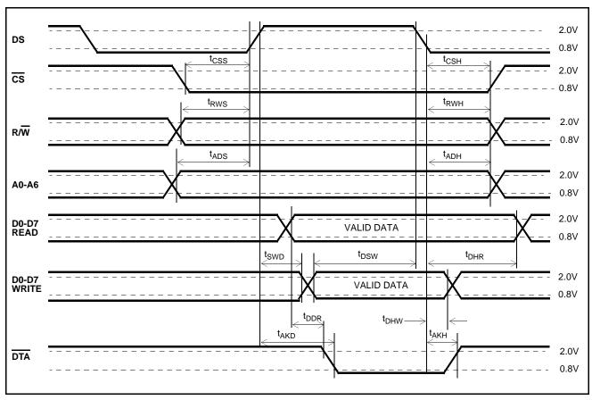
Figure 28 - Motorola Non-Multiplexed Bus Timing
