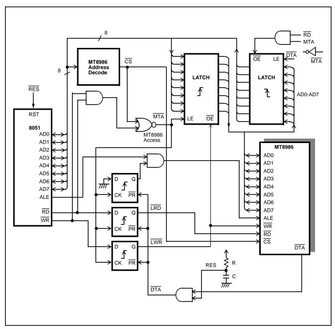
Figure 14 - Interfacing the MT8986 to the 8051 Microcontroller
