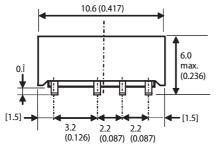
Tolerance of lead pitch is  $\pm 0.15$ mm (0.006inch) Other tolerances ±0.3mm (0.012inch)
