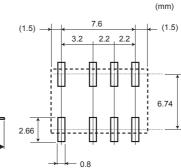
Tolerance of lead pitch is  $\pm 0.15$ mm (0.006inch) Other tolerances  $\pm 0.3$ mm (0.012inch)
