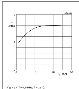
Fig.4 Transition frequency as a function of collector current.
