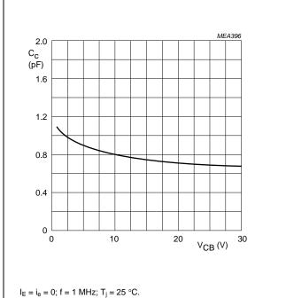
Fig.3 Collector capacitance as a function of collector-base voltage.
