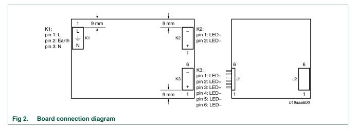
If a galvanically isolated transformer is used, it should be placed between the AC source and the dimmer/demo board. Connect a user defined LED (string) to connector K2 as shown in <a href="Figure 2">Figure 2</a>. Note that the anode of the LED (string) is connected to the bottom side of this connector.
