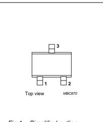
Fig.1 Simplified outline (SOT323; SC-70) and pin configuration.
