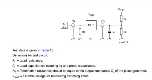
Fig 9. Test circuit for measuring switching times
