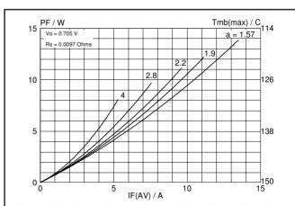
Fig.6. Maximum forward dissipation  $P_F = f(I_{F(AV)})$  per diode; sinusoidal current waveform where a = form factor  $= I_{F(RMS)} / I_{F(AV)}$ .
