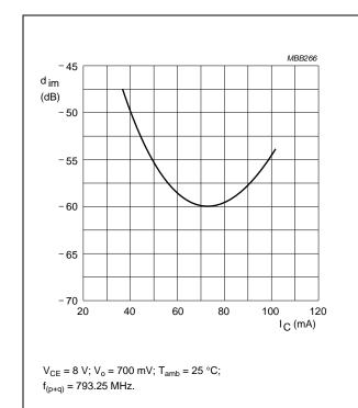
Fig.10 Intermodulation distortion as a function of
