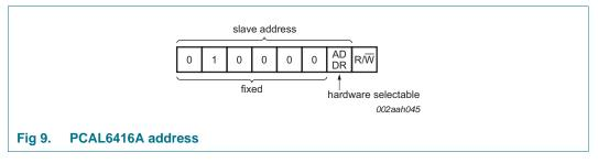
ADDR is the hardware address package pin and is held to either HIGH (logic 1) or LOW (logic 0) to assign one of the two possible slave addresses. The last bit of the slave address (R/W) defines the operation (read or write) to be performed. A HIGH (logic 1) selects a read operation, while a LOW (logic 0) selects a write operation.
