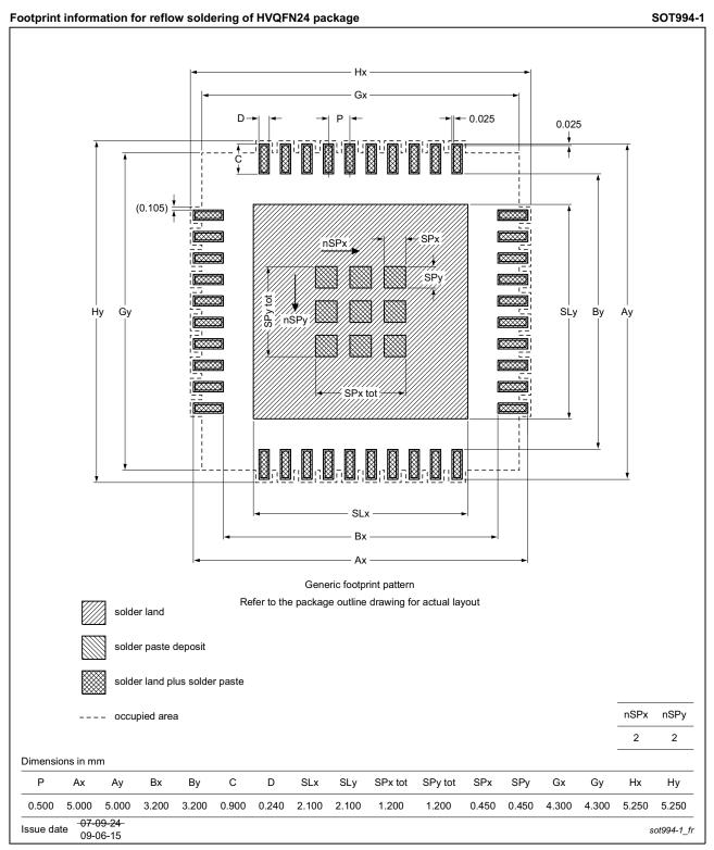
Fig 46. PCB footprint for SOT994-1 (HWQFN24); reflow soldering
