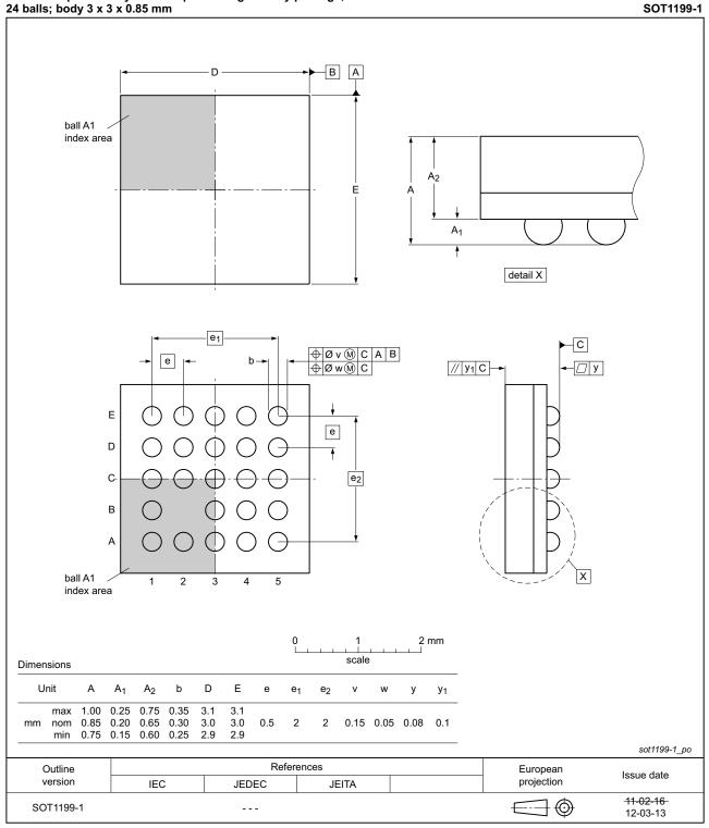
VFBGA24: plastic very thin fine-pitch ball grid array package; 24 balls; body 3 x 3 x 0.85 mm
