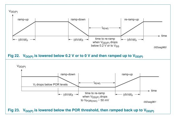
The two types of power-on reset are shown in Figure 22 and Figure 23.
