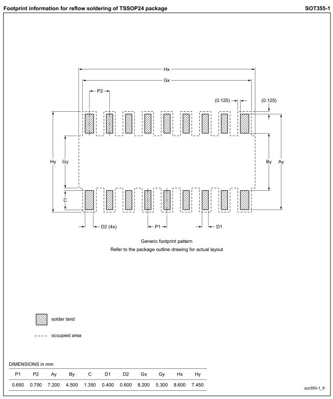
Fig 45. PCB footprint for SOT355-1 (TSSOP24); reflow soldering
