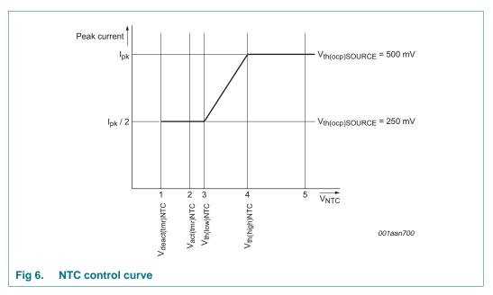
When the voltage on the NTC pin exceeds  $V_{th(high)NTC}$  (see Figure 6 (4)), the converter delivers nominal output current. When the voltage is lower than this level, the peak current is gradually reduced until  $V_{th(low)NTC}$  is reached (see Figure 6 (3)). The peak current is now half the peak current of nominal operation. When  $V_{act(tmr)NTC}$  is passed (see Figure 6 (2)) a timer starts to run to distinguish between the following situations:
