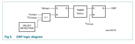
The value of  $t_{on(high)}$  depends on the capacitor connected to the TONMOD pin. An open or shorted TONMOD pin sets  $t_{on(high)}$  to 15 µs (see Section 8.4.6 and Table 6).
