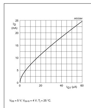
Fig.7 Drain current as a function of gate 1 current; typical values.
