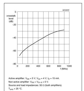
Fig.19 Crosstalk as a function of frequency: Output level of non-active amplifier related to output level of active amplifier; typical values.
