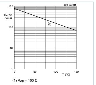
Fig. 13. Critical rate of rise of off-state voltage as a function of junction temperature; typical values
