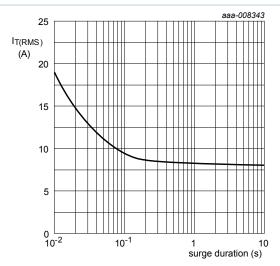
f = 50 Hz;  $T_{mb} = 135 \,^{\circ}\text{C}$
